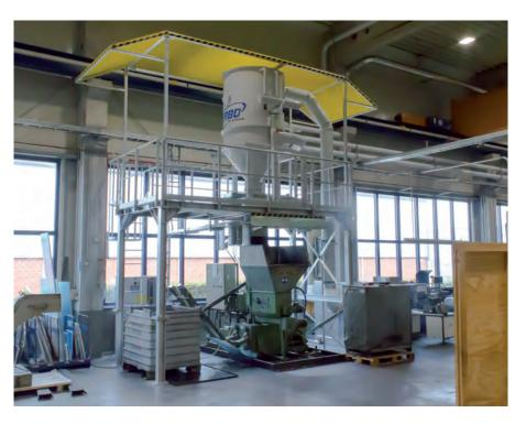
Our central extraction system makes it possible to automatically separate alloys in aluminum swarf, or to automatically separate metal and aluminum swarf.
